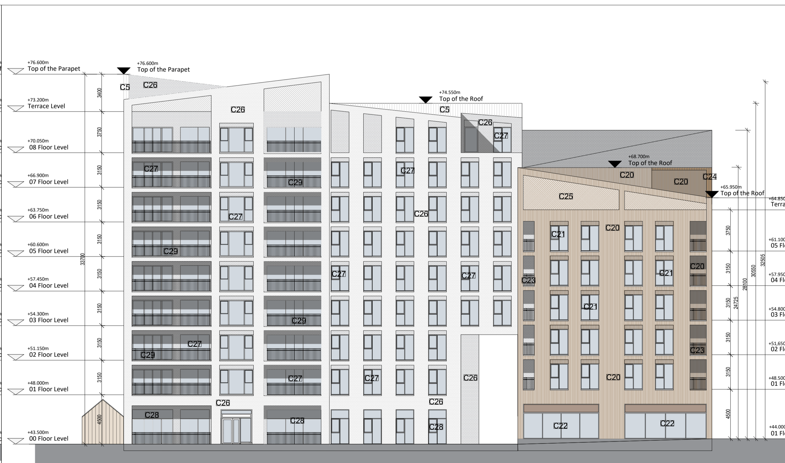
BLOCK 8 WEST ELEVATION 1:200@A1
